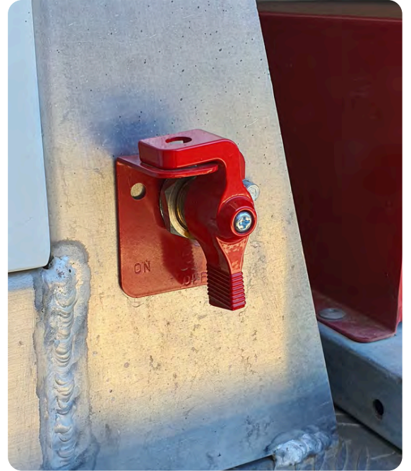
Engage Battery Isolator to avoid unwanted battery discharge
