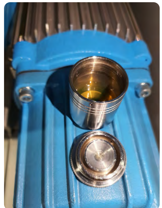
The Reservoir only needs to be filled half way
