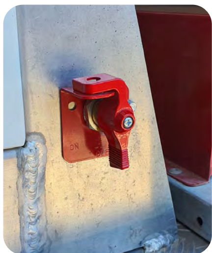
Battery Isolation Switch
